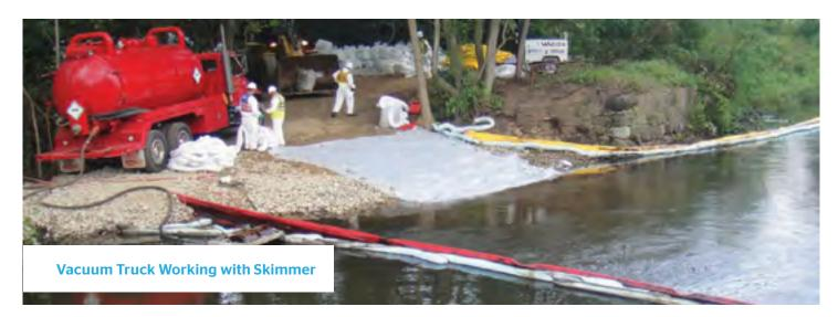
The skimmer can be connected to a vacuum truck to suck out recovered oil. The drums may be driven by the compressed air provided by the trucks braking system.
